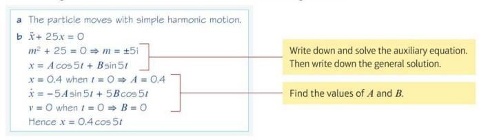
c Period of motion is  $\frac{2\pi}{5}$  seconds  $\dot{x} = -2\sin 5t$ , so maximum speed =  $2 \text{ m s}^{-1}$ .
